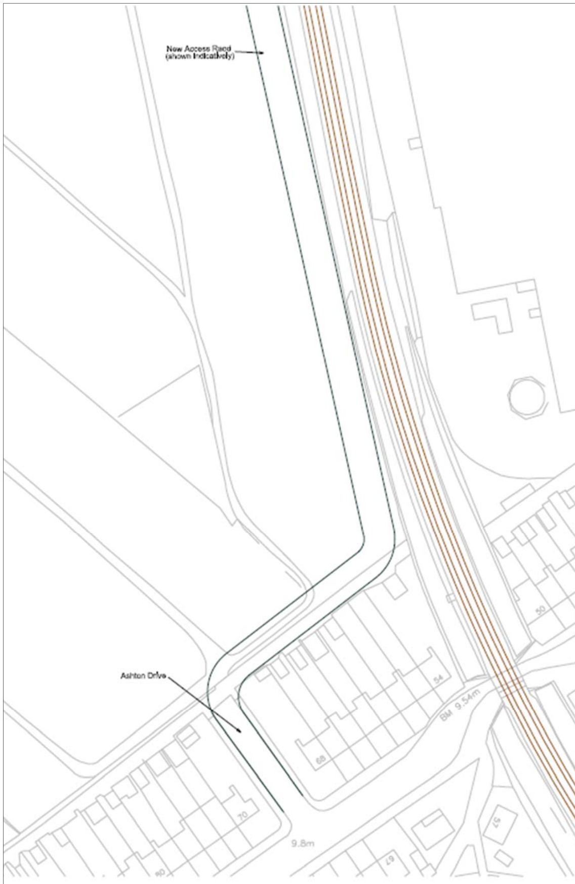
Figure 2-7: Ashton Gate station – layout Option 2b (new access road via Ashton Drive)
